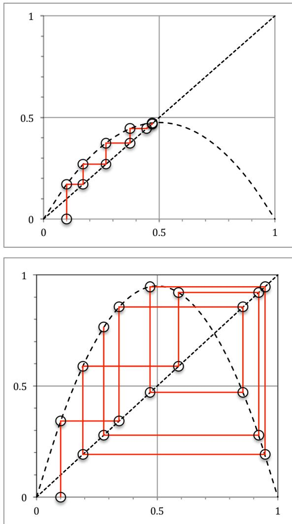
Figure 2. Examples of graphical integration of recurrence equation (2) for various values of growth parameter  $r$ : 1.9 (top), 3.8 (bottom)
