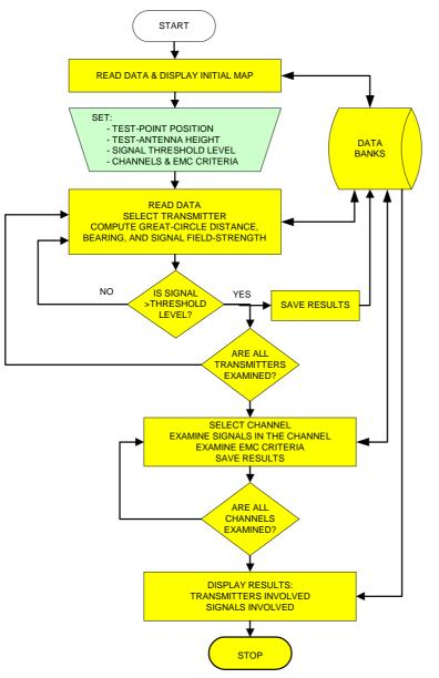
*Figure 8A*-Signal environment: flow diagram (simplified).
