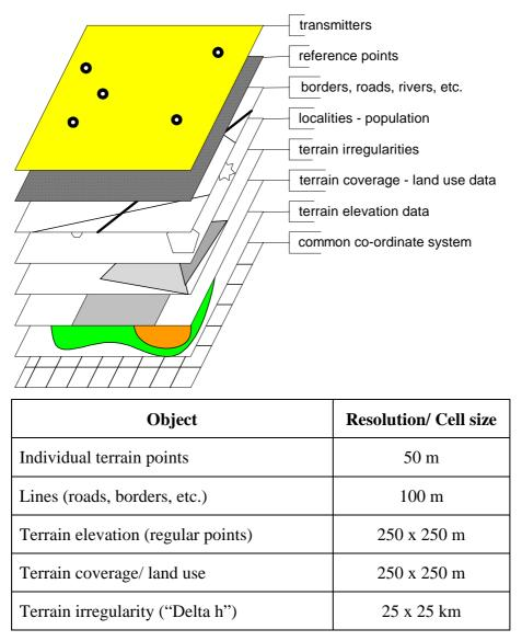
*Figure 2-Geography-related data use common co-ordinate system. Data from maps in various scales can be automatically adjusted and superimposed*
