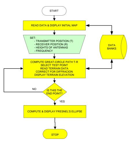
*Figure 6A*- *Terrain elevation profile: production process (simplified diagram). The yellowmarked tasks are performed automatically*
