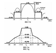
Spectrum masks for WiFi – examples of the projection of multidimensional signal solid onto the Frequency-Power plane
